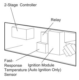
Fig. 25: Control Box Component Locations Models 135 & 180
